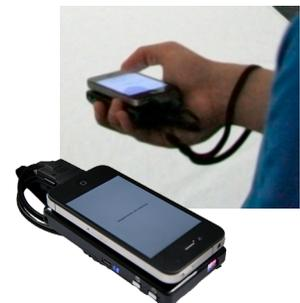
**Figure 5: The prototype hardware. An iPhone4 affixed on top of a SHOWWX+ laser projector, connected via a cable.**
