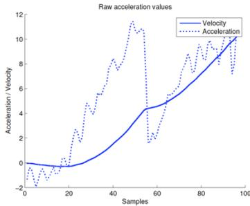
**Figure 6: During the swing phase raw accelerometer values are logged and then integrated to compute the current velocity of the device which is applied as impulse to the bowling ball.**
