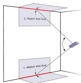
**Figure 4: The user lines up two calibration pictures that allow the system to compute the distance to the wall.**
