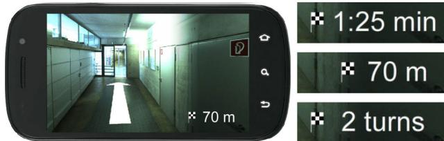
Figure 2. Left: Prototype showing a navigation arrow as overlay to the video image. Right: Variants for displaying the distance to the goal
