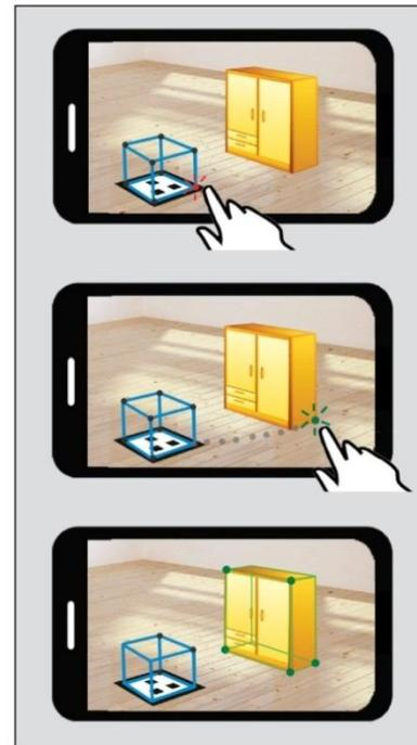
**Figure 4: Direct Interaction - Point out to our system the correspondences between the unit box corners to those of the object. The system computes the object size automatically.**
