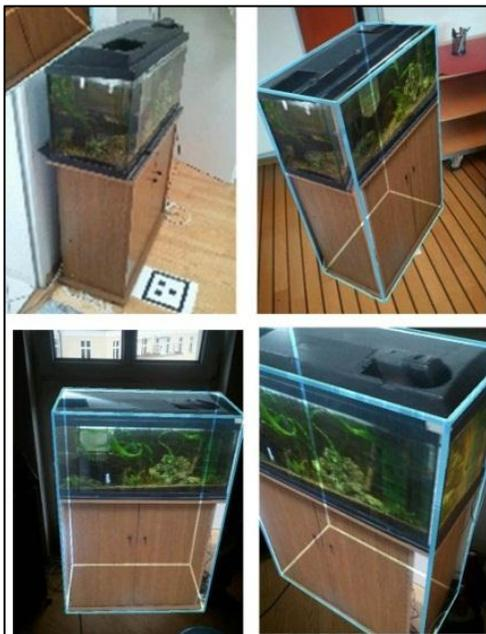
Figure 7: The real aquarium (top left) was measured using the “model manipulation” method and then textures were automatically extracted by the mobile app in real time. The remaining images show the same aquarium virtually placed in different environments and viewed from various perspectives.
