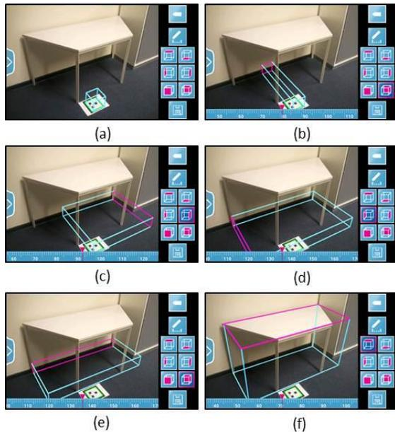
**Figure 3: Android smartphone with model manipulation based interface for visual metrology. The user selects faces (b–f): rear, right, left, front and top, in order to directly manipulate a virtual bounding box to fit its view in the image. The control-cube provides the object size and position.**
