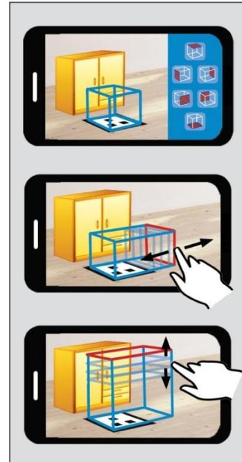
**Figure 2: Model manipulation with feedback interaction: Here we allow the user to choose the specific face of the bounding box to moved. Then a simple swipe of the finger either left/right extrudes the box along that face. Since the actual size of the 3D model is internally maintained, the visual overlay provides feedback in the image as to its fit to the object. When satisfied, this directly provides the size and position of the object/furniture with respect to the marker.**
