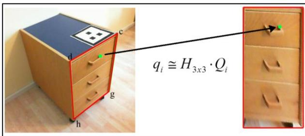
Figure 6: A homography is used to find the corresponding pixel  $q_i$  on the source image and map it to the texture  $Q_i$ .
